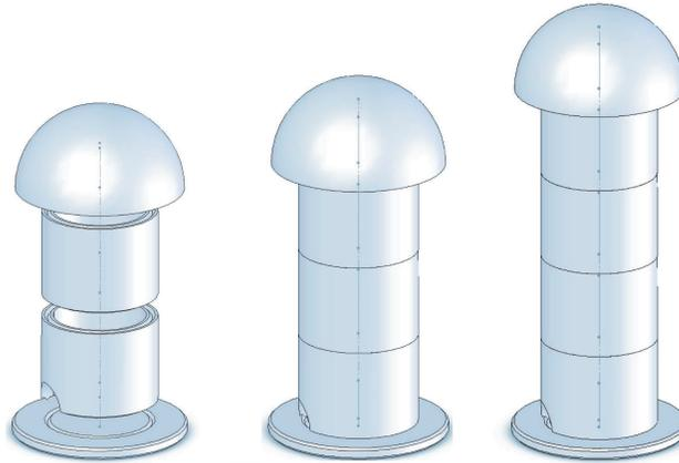
Fig. 6. CAD Model of Starling Bird Feeders [32], [33], [36], [46]
