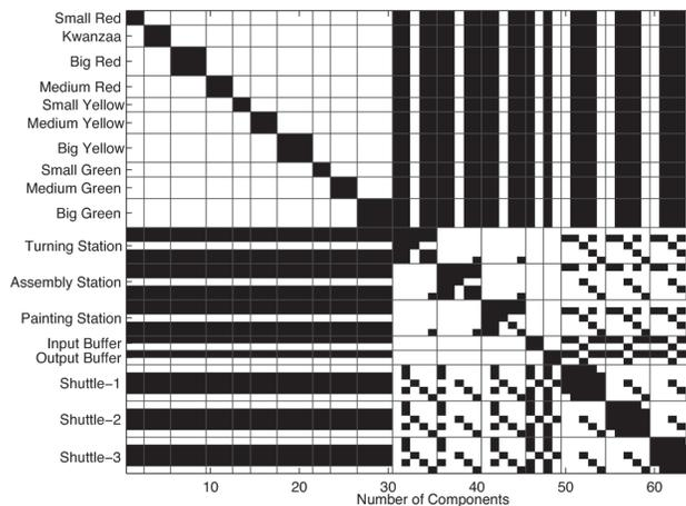
Fig. 11. Starling Manufacturing System Production Design Structure Matrix [33], [36]
