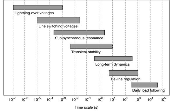
Figure 10: Timescales of Physical Power Grid Dynamics [5]
