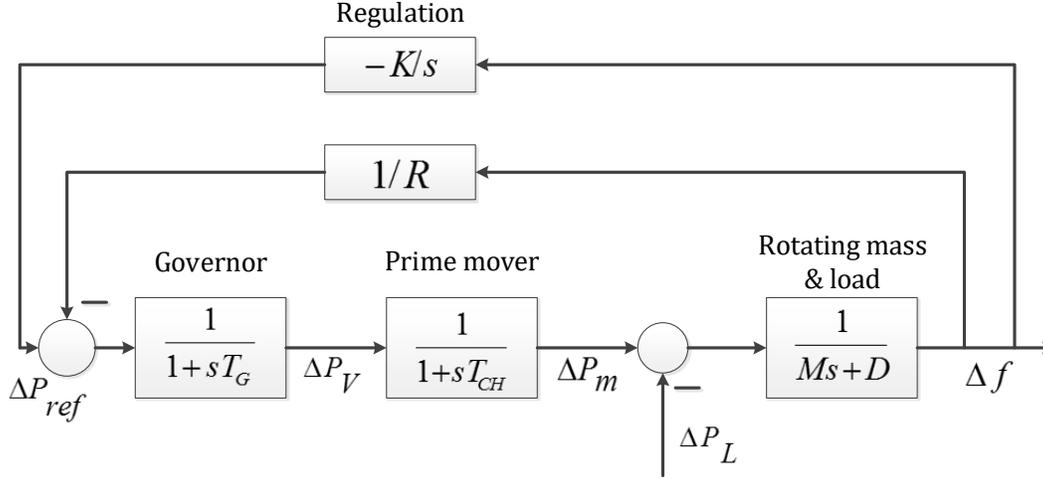
Figure 19: Power System Automatic Generation Control [9]
