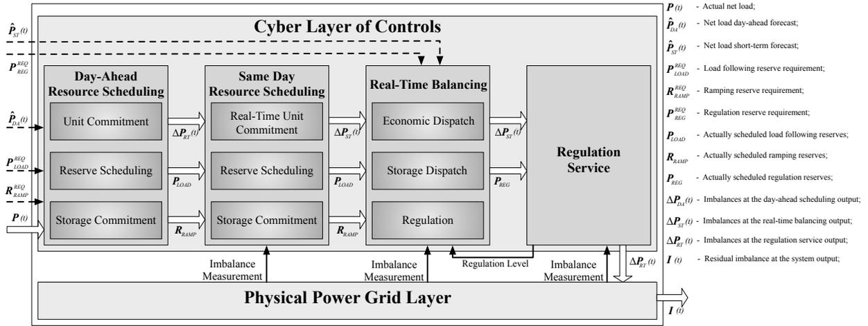
Figure 13: Architecture of the Electric Power Enterprise Control System (EPECS) Simulator Customized for ISO New England Operations
