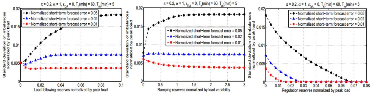
Figure 31: Impact of VER Short-Term Forecast Error on Power System Imbalances [11]
