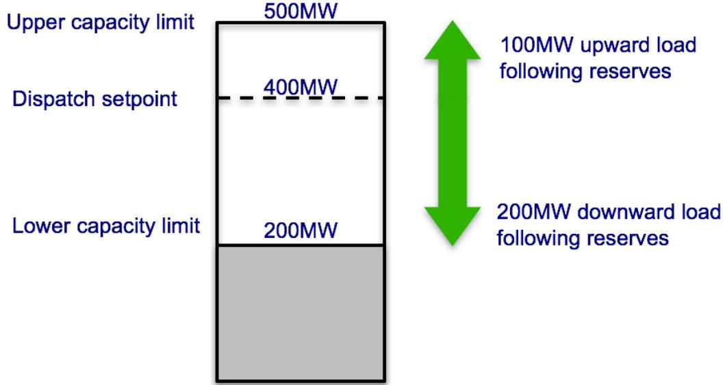
Figure 15: Load Following Reserves Example: A hypothetical generator with a maximum capacity of 500MW, and minimum capacity of 200MW, and dispatched to 400MW provides 100 MW of upward load following reserves, and 200 MW of downward load following reserves.
