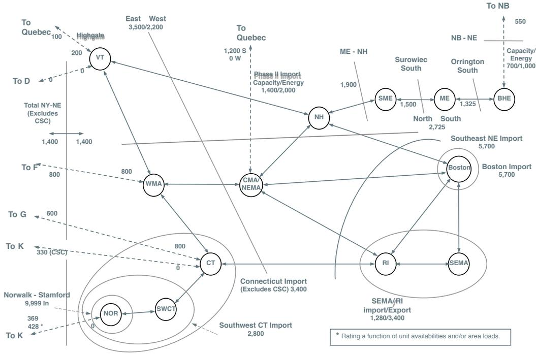
Figure 20: Topology of the ISO-NE Zonal Network Model [10]
