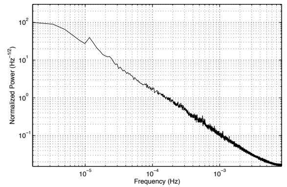
Figure 12: Wind Power Spectrum [7].
