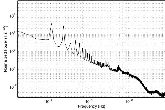
Figure 9: Normalized Power Spectrum of Daily Load (Data from [4]).
