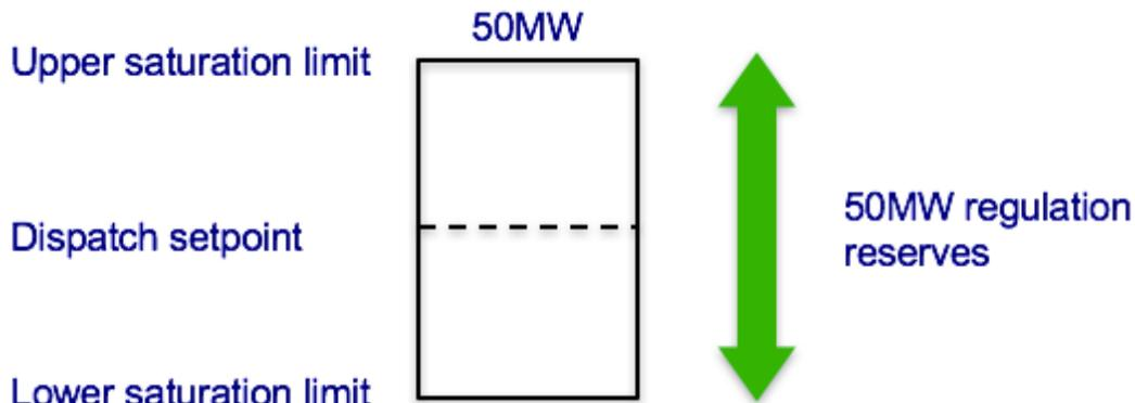
Figure 17: Regulating Reserves Example: A generator with saturation limits of 50MW on its automatic generation control also provides 50MW of regulation reserves.
