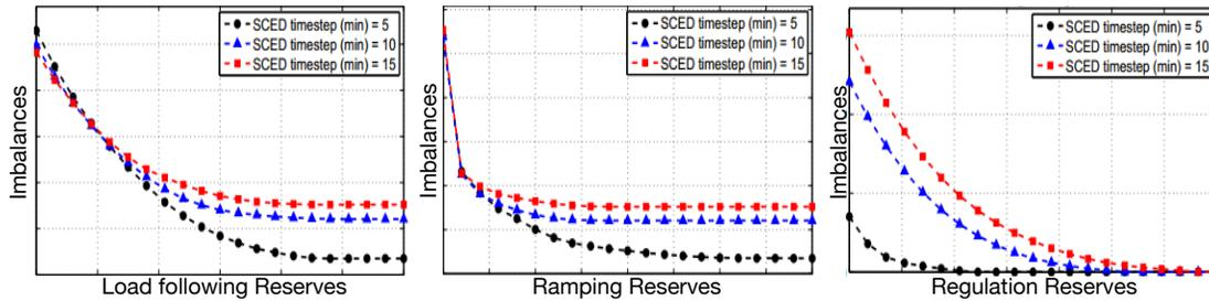
Figure 8: Operating Reserves Assumption 4: Non-dependence of Imbalances on Power System Operator Decisions & Control
