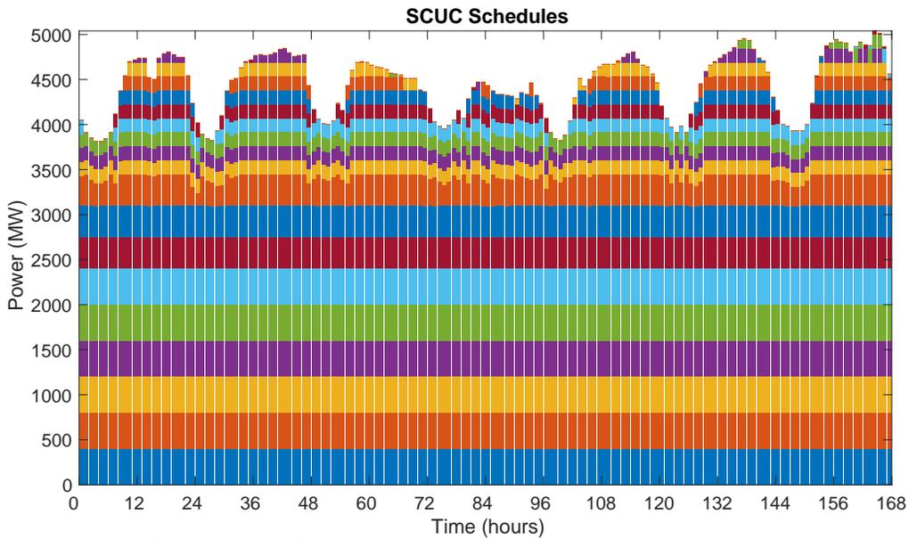
Figure 22: EPECS Simulator Output: The Security Constrained Unit Commitment Schedule
