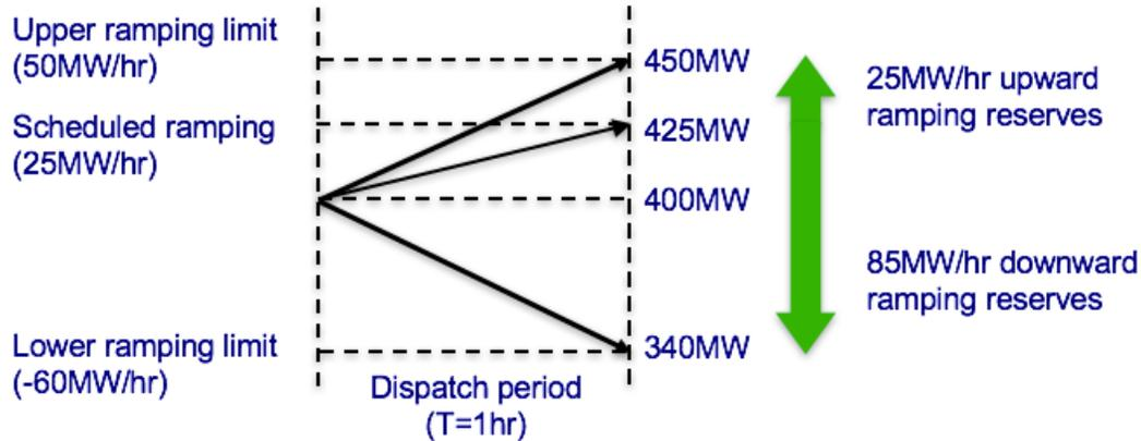
Figure 16: Ramping Reserves Example: A hypothetical generator with maximum ramp up of 50MW/hr and maximum ramp down of 60MW/hr is scheduled to ramp from 400MW to 425MW in one hour. It provides 25MW/hr of upward ramping reserves and 85MW/hr of downward ramping reserves.
