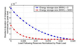
Fig. 9 The relative trade-offs of utilizing normalized loadfollowing reserves versus energy storage on the normalized standard deviation of imbalances [48].
