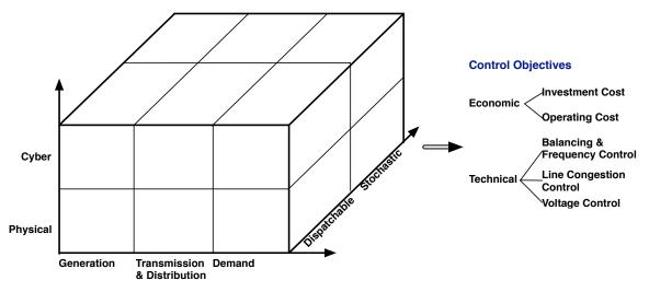
Fig. 1 The power grid is taken as a cyber-physical system composed of an energy value chain with dispatchable and stochastic elements that must fulfill certain technical and economic objectives [32]
