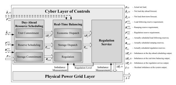
Fig. 2 A conceptual model of the power grid enterprise control simulator [34].
